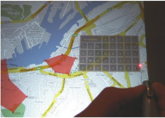
**Figure 5:** *Tabletop interaction II: a new name for an object (here a new obstacle) is entered by means of a virtual on-screen keyboard Pen Grabber and sent through the Quartz Java Bridge is processed to create, edit, or remove items. Currently, the library includes items for obstacles, routes, and units. Items are displayed on Google Maps.*
