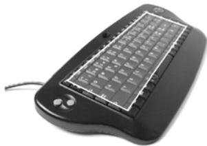
**Figure 1.** Touch&Type™ (1<sup>st</sup> generation prototype); the mouse buttons are shown left; the touch sensitive area is framed.
