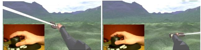
**Figure 3 Basic movements: Left deflection of the device moves the sword to the left (left); right deflection of the device moves the sword to the right (right).**
