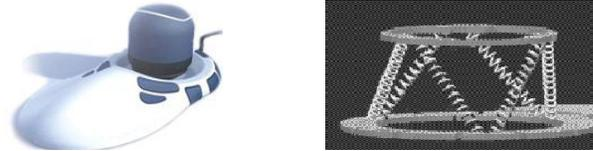
**Figure 1** The SpaceCat 6DOF device (left). The handle is suspended with inductive metal springs (right); these springs also serve as sensors [1].
