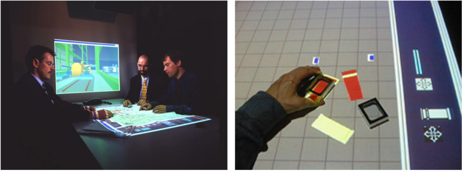
Fig. 5. The BUILD-IT system: Collaborative production plant layout combining digital, physical, and printed media (left); multi-pointer interaction of a furniture scenario (right)
