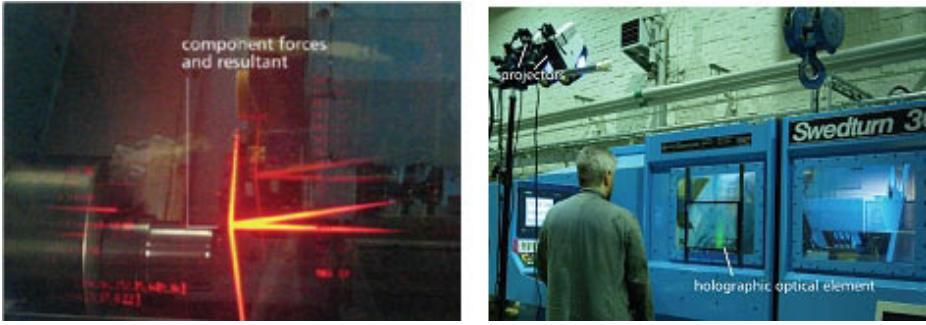
Fig. 2. The operator views the machine operation through the holographic optical element (HOE), which is illuminated with stereoscopic images from the projectors driven by a PC. The setup allows 3D annotation to appear in the workspace, augmenting the operator’s view of the process with relevant information [33].
