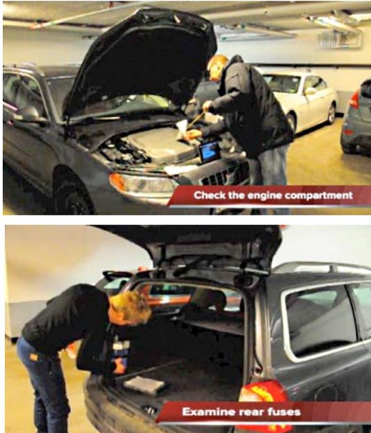
**Figure 8: Tasks evaluated: SEMarbeta used for checking oil in the engine compartment (top) and voice-only used for examining rear fuses (bottom).**
