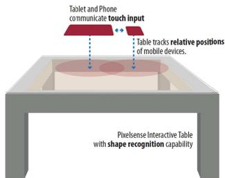
**Figure 3.** The first generation MochaTop prototype.
