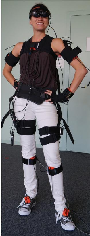
**Figure 1:** User wearing the proposed AR setup consisting of an inertial motion capturing suit and see-through HMD.
